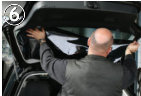
Now take off the prepared film from the outside and put it on the wet car window. As long as there is a water layer between the tinting film and the glas, you can shift the film as you like. Moisten the film again from inside.
