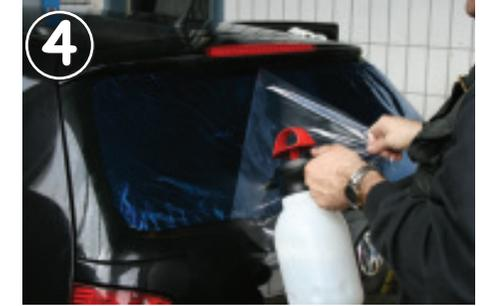
Fit the film perfectly to the glas. Remove the liner from the tinting film by sticking two small stripes of adhesive tape in one corner to either side of the film and then pulling the two stripes apart from each other. This will pull the liner from the tinting film. Immediately spray lots of water on the adhesive side of the film while pulling off the liner.
