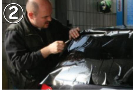
Lay the film on the outside of the wet window. The protection layer of the film (liner) shows towards yourself. See step 4 how to find the liner. Cut around the glas and leave around 2-3 cm overlapping on each side of the car window. The film will later shrink when you heat it up. The precise cut will be done later.
