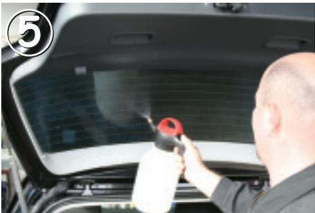
Also moisten the inner side of the car window with lots of the water. The more fluid is on the glas the easier is the installation.
