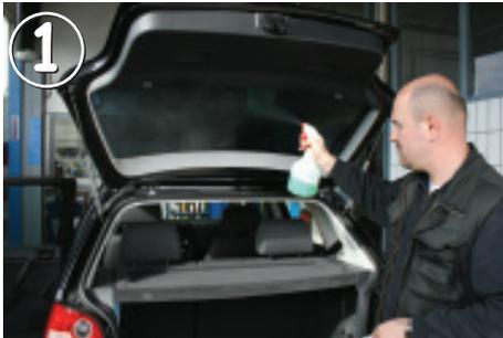
Free the car windows with a household glas cleaner from any dust and grease. For the installation, we recommend distilled water with 3-5 drops of dish-washing liquid per litre. This will break the water's surface tensions. Fit the film to the side windows first, as they are usually easier to tint. Be sure to leave enough film for the rear window.
