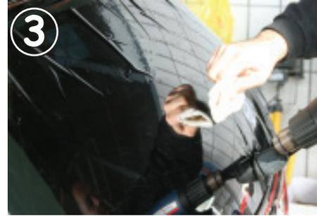
On curved windows, the film will not lay flat, but rather shows folds. Use a heat gun to fit the film to convex glas. Pay attention to the temperature recommendations on the packaging! The film will shrink in horizontal direction (left-right) when heated. Heat the folds and push them flat with the scraper. Larger folds split into smaller ones until the film will be free from folds.
